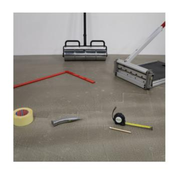
face up. When cutting the vinyl plank, mark the line and use the knife to make a firm cut in the surface. It is recommended to wear gloves. We recommend staggering the rows by at least 30 cm so that the short edges are not in the same line.
