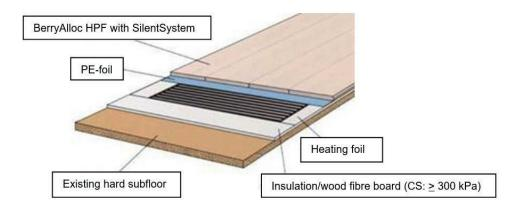
When installing BerryAlloc HPF without underlay the insulation boards must have a compressive strength (CS) of min. 120 kPa (according to EN 16354:2018).
