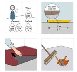
The subfloor has to be even (maximum deviation of 3 mm per m or 1 mm over a length of 20 cm). If the indicated deviation is exceeded, the subfloor must be levelled out with a suitable filler. Smoothen sharp edges and fill any holes. This is important because an uneven subfloor can cause squeaking noises or may telegraph through the new floor, resulting in an unsightly surface and causing excessive wear on high spots or indentation on lower spots.
