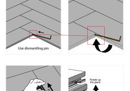
When a plank is locked, it is not possible to simply remove it by hand. Use the 5G® dismantling pin to dissassemble the planks. Insert the pin in the click system and push it until reaching the end of the plank. Lift up the plank, for your safety, use protective clothing: gloves, dust mask, protective glasses.
